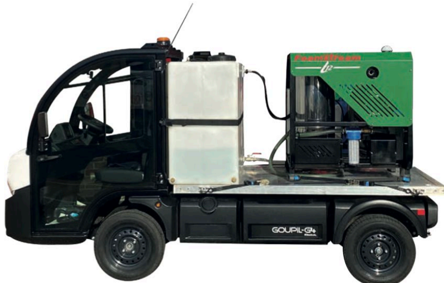
Figure 8 - Foamstream L12 with Bowser on the Bradshaw G4 Flatbed Electrical Van
