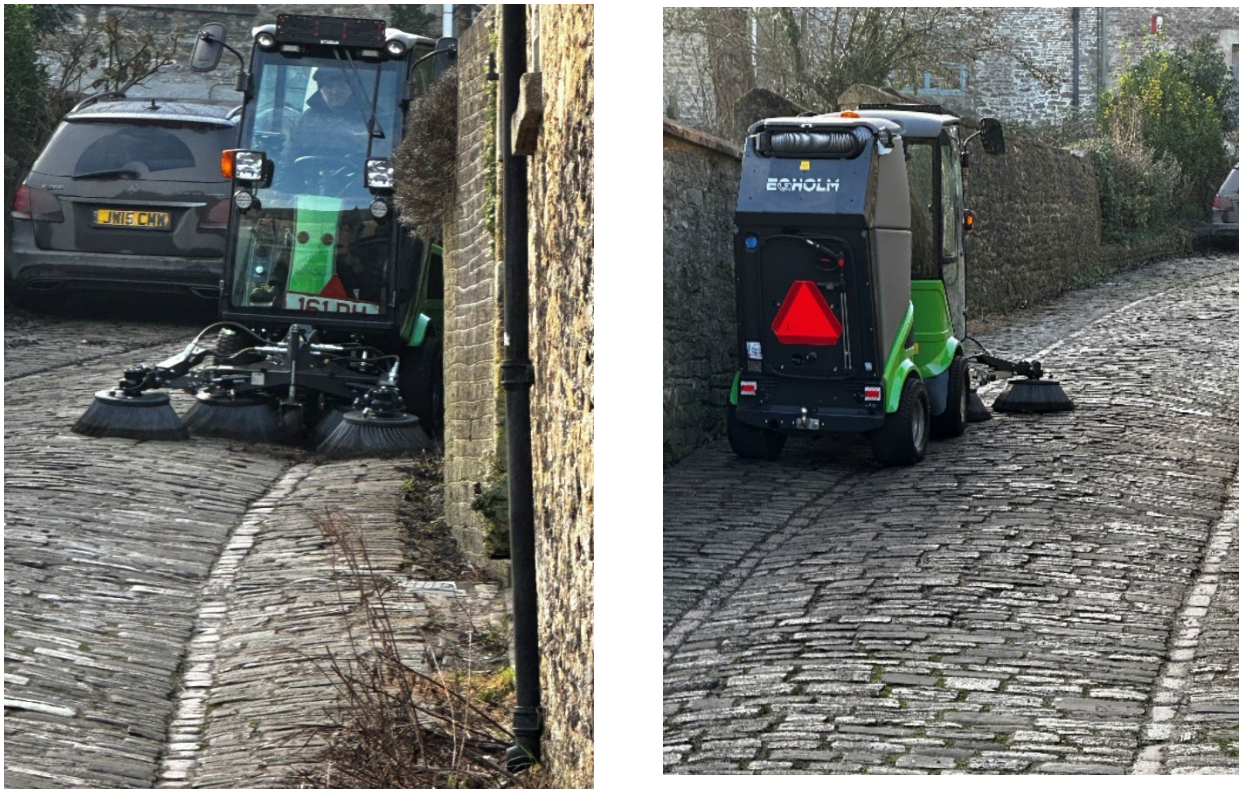
Figures 17 and 18 - The sweeper managing to clear moss/lichen on the steeper cobbles of Gentle Street without struggling with the slope or damage to the cobbles.
